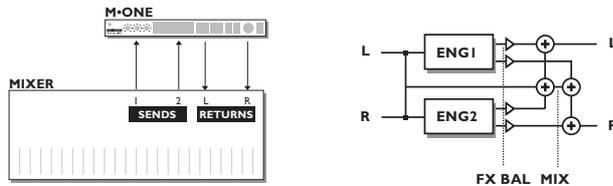
This is the routing to use if you wish to use the M•ONE as two independent effects processors. Left Input is sent to Engine 1 and right Input is sent to Engine 2. The four FX Outputs are summed to two channels.
