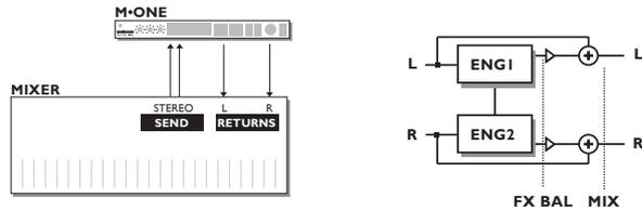
In the Stereo Linked Routing the Engines perform the exact same effect with synchronized parameter settings. Left I/O are used for Engine 1, Right I/O are used for Engine 2. When switching to Stereo Linked Routing the Engine 1 settings are forced into Engine 2.
