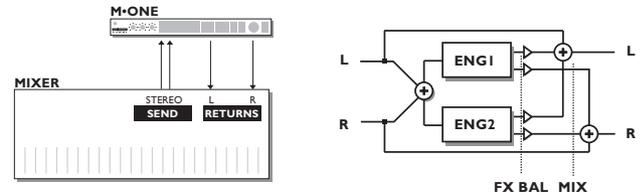
The Parallel routing sums left/right Inputs, and both Engines are fed with the exact same signal. As illustrated the unprocessed dry signal is mixed with the processed signal into two channels via the Mix parameter.
