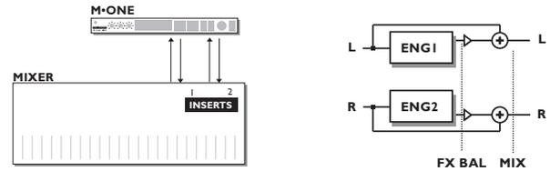
In the Dual Mono routing, the two Engines are totally independent, meaning mono in/mono out of each Engine. Left I/O are used for Engine 1, Right I/O are used for Engine 2.
